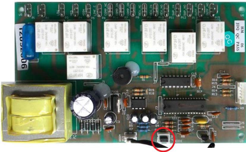
Retire o "Jump" do Conector P17.
